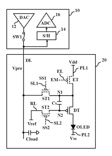
TFT DT, as expressed by the following Equation 3. In Equation 3, "Cload" represents load applied to the data line DL, namely, the parasitic capacitance of the data line DL.
